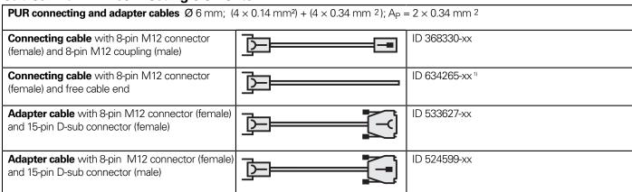
A<sub>P</sub>: Cross section of power supply lines
