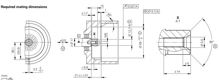
Tolerancing ISO 8015 ISO 2768 - m H < 6 mm: ±0.2 mm
