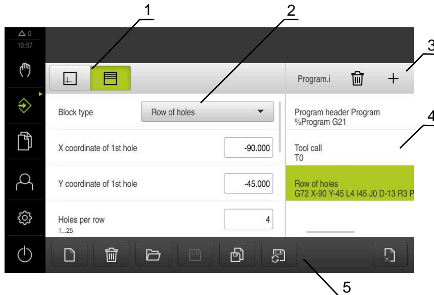
Figure 58: Example of a program in the Programming operating mode
