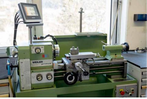
Altogether, eight conventional, manually operated machines were converted as part of the retrofit.
